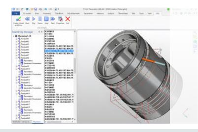
Associativity is provided between the T–FLEX CAD model and T–FLEX CAM machining in all machining operations.
