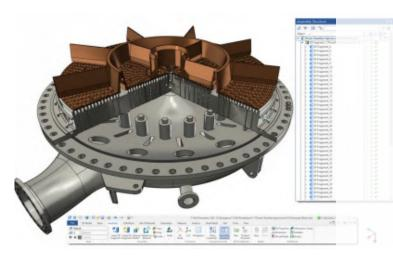
This functionality helps you for example associate parts in a way that allows the change of one part to drive changes in associated parts. Any thing in T–FLEX can be related to anything else. Variables can be assigned at any time for component names, visibility, material, any numeric or text attribute of any entity. They can then be processed with any algebraic or logical expression to control the behavior of the design.
