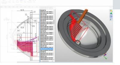
When a new tool is created with T-FLEX CAM punching module, the definition includes all of the information necessary to provide the greatest control over tool use. The tool-path can be reviewed at any time with tool-path simulation. Tool hits can be stepped through one at a time, by tool sequence, or full simulation. T-FLEX CAM provides automatic tool-path optimization to minimize CNC machine run-time.
